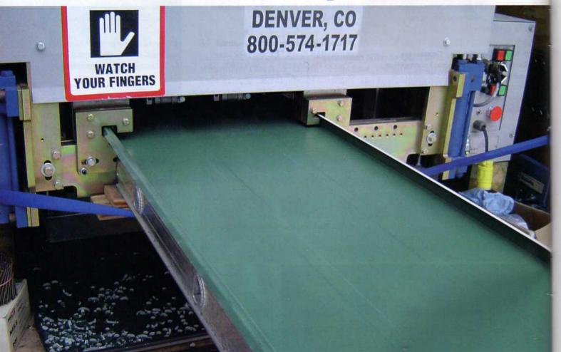
When working with single lock standing seam roofing, the ability to manufacture double male panels is useful for several situations.
