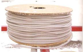
PREVENTING OIL CANNING » Three-eighths-inch backer rod can be applied to the center of roof panels starting and ending about 8 inches from each end of the panel. The backer rod is attached every 5 feet or so with a small piece of duct tape, which will adhere well to steel in almost any weather condition. / Backer rod costs about 3 cents per linear foot and can be applied very quickly. It serves as relatively inexpensive insurance against the appearance of excessive oil canning.
